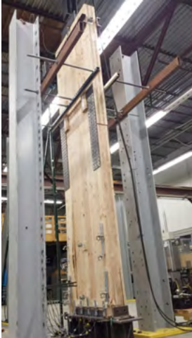
A two-storey vertically prestressed CLT shear wall undergoing testing at Washington State University, one of eight universities and industry bodies collaborating in a programme funded by the US National Science Foundation to develop CLT shear wall systems suitable for regions of high seismicity.
