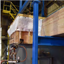
A full-scale fire test for glulam beam to column connectors, testing the connector to meet a minimum of 1hr fire resistance rating.
